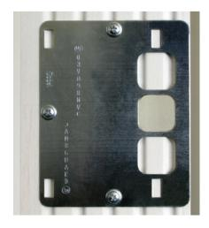
JambGuard is a steel reinforcement plate that is installed to the backside of the jamb, at the deadbolt location, on a single prehung door. This provides greater strength to the jamb against break-in force.
