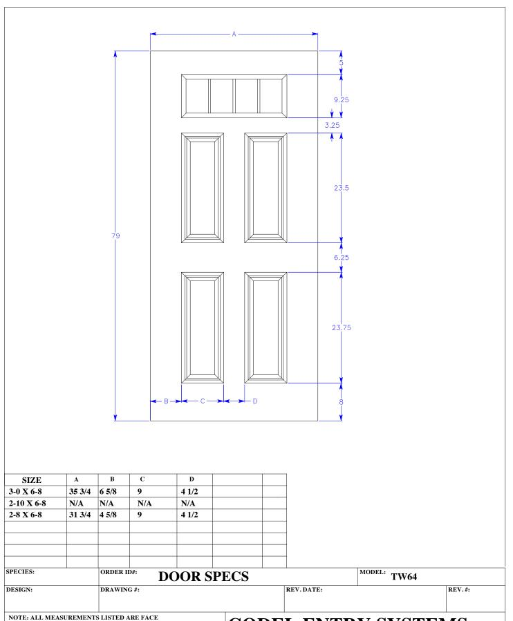
NOTE: ALL MEASUREMENTS LISTED ARE FACE DIMENSIONS.UNLESS OTHERWISE NOTED, ALL UNITS ARE INCHES. TOLERANCE = ±1/32" **CODEL ENTRY SYSTEMS** ±1/32" DRAWN BY: DRAWN DATE: PAGE #: 1 OF 1
