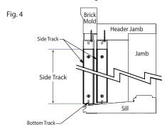
5. The screen should be installed top first into header track, then positioned over the bottom track on sill.
